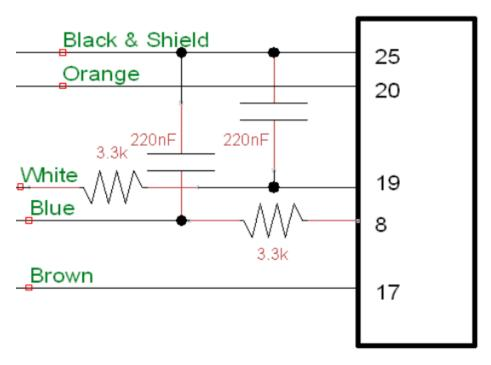
\*Note - When the external PTT line is engaged, the BCR repeater will transmit with the settings configured in the User 1 slot. Refer to the BCR User manual (Page 8).
