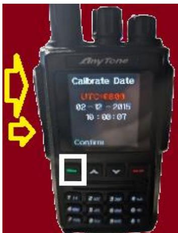
b.) With the radio off, Push the PTT button, and the Button directly below it. That button is also called the PF1 Key. Then While holding both buttons, Turn the power on, and wait for the radio to boot. Don't release them yet.
